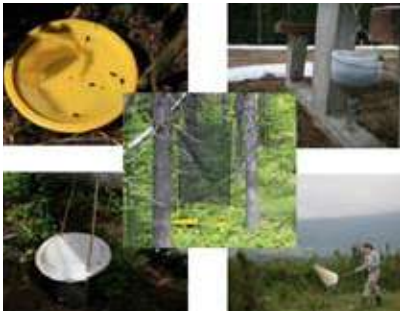
Traps used in the Standardized Sampling Program: pan trap (top left), Berlese funnel (top right), flight intercept trap (centre), pitfall trap (bottom left), sweep netting (bottom right)
