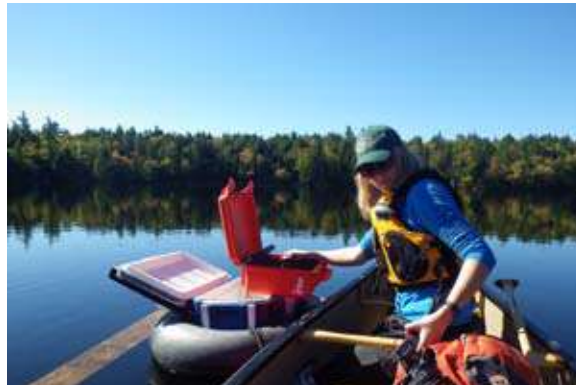
S. Klapstein checking on her floating equipment for measuring UV, PAR and temperature in Big Dam East and Big Dam West
