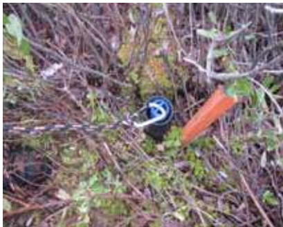
Observation well at Heber Meadows with bailer inserted for water sample collection
