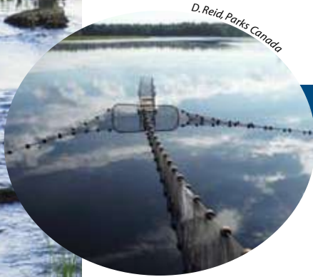
The Turtle-safe fyke net deployed at Loon Lake, Kejimikujik
