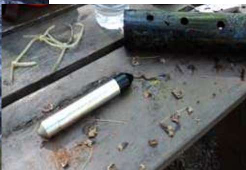
HOBO water level logger removed from its protective PVC housing
