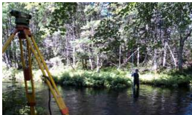
The exact depth of the submerged water level logger is measured using precision survey equipment
